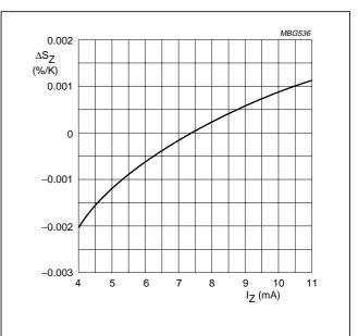
Fig.3 Temperature coefficient change as a function of working current; typical values.
